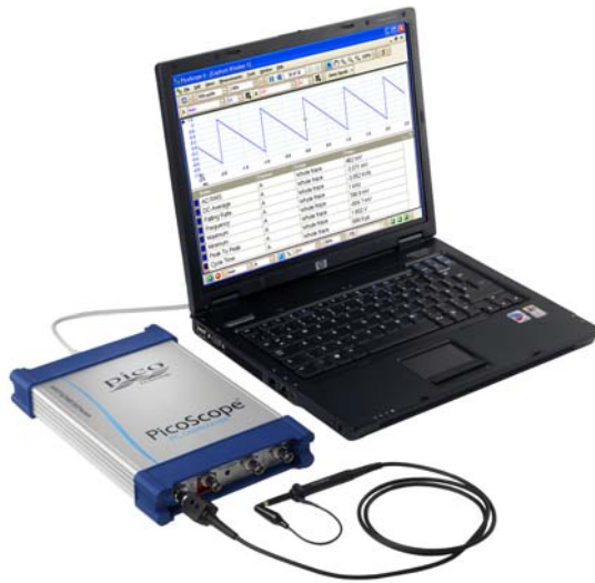
Photo Caption: The PicoScope 5000 series API lets you control the world's fastest USB PC Oscilloscope from your own software.
